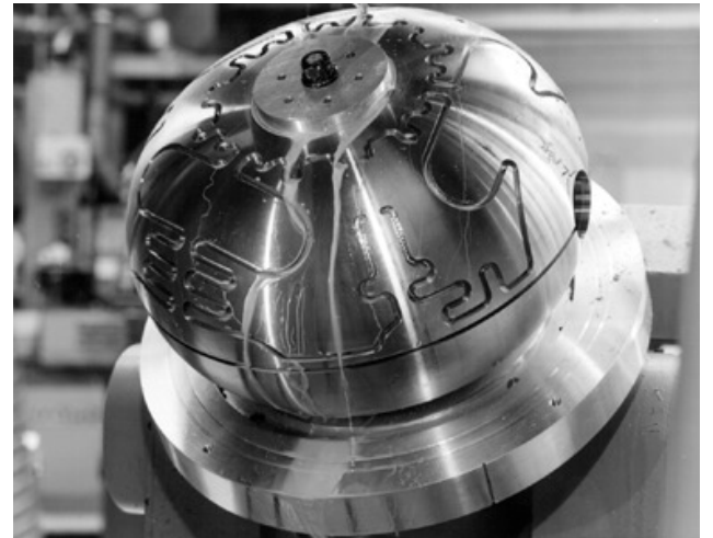
Figure 10 RF cavity during machining of water cooling grooves.
