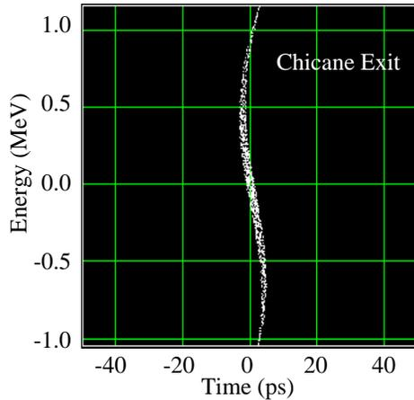
Figure 3. Longitudinal phase space after the chicane when the beam is linearized and compressed.
