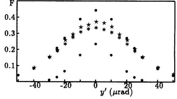
Figure 2.  $F(y')$  scan for  $x'=0$ . Ideal crystal: (o) first-pass and (●) overall efficiencies. Imperfect crystal: overall efficiency with  $t=1 \mu\text{m}$  (\*) and  $t=50 \mu\text{m}$  (x).
