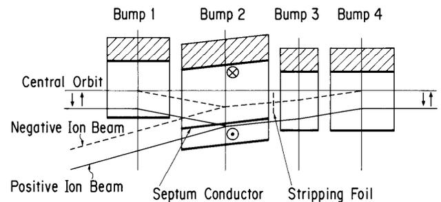
Figure 1. New injection system for the booster
