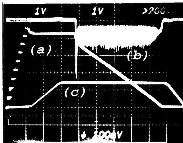
Figure 4. Helium acceleration in the main ring: (a) a helium beam intensity during a cycle, (b) a slowly extracted intensity and (c) a main magnet field pattern.
