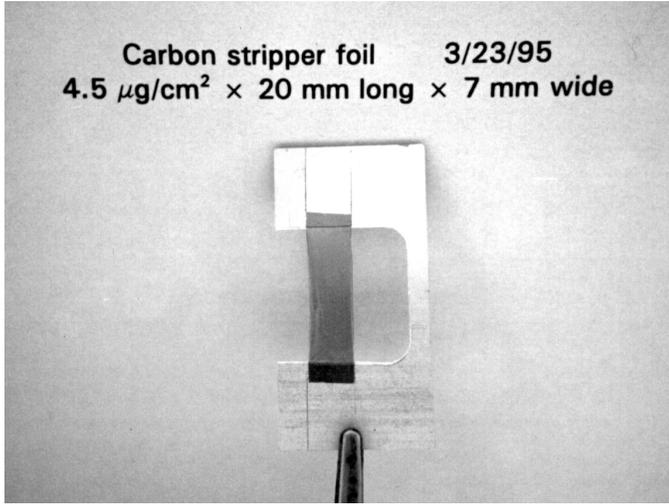
Figure 1. The  $4.5 \mu\text{g}/\text{cm}^2$  carbon stripper foil with two unsupported edges. The width of the foil is 7 mm.
