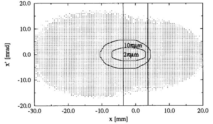
Figure 2. The usable emittance at the injection energy (7 MeV) for the  $2\pi \mu\text{m}$  and  $10\pi \mu\text{m}$  cooler acceptance. The emittances appear larger than they are because individual particles have different closed orbits. The vertical lines indicates the location of the stripper foil and the shaded area the CIS acceptance.
