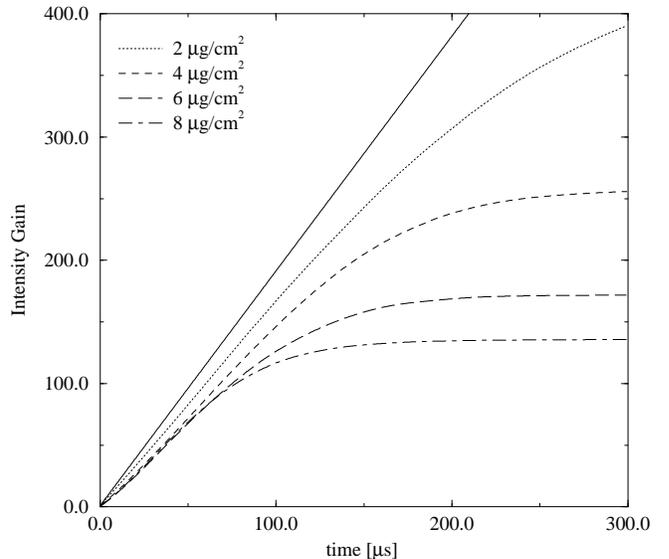
Figure 3. The intensity gain of 7 MeV protons plotted vs. the pulse length from the RFQ and for different foil thicknesses. The acceptance of the Cooler injection channel was  $10\pi \mu\text{m}$ . The solid line shows the gain calculated without energy loss or scattering at the foil.
