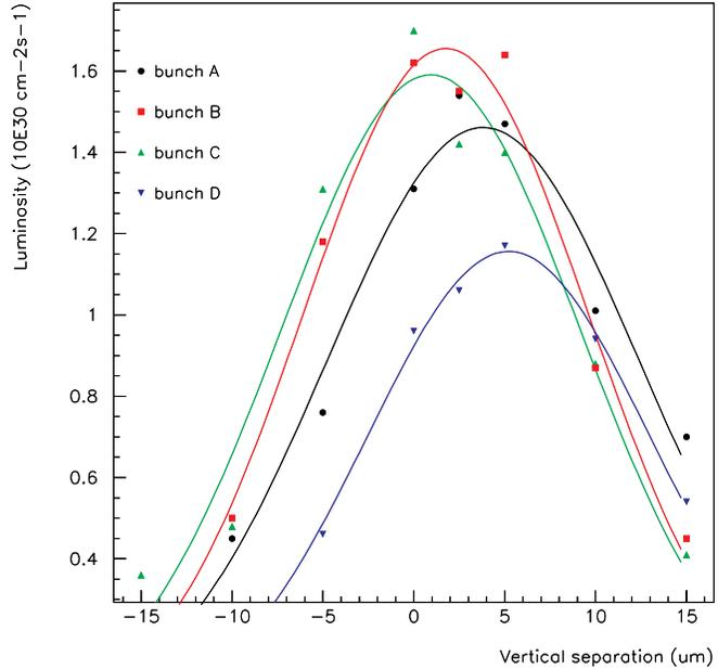
Figure 2. Plot of a Vertical Luminosity Scan of Bunch Trains derived from the LEP Measurement Database
