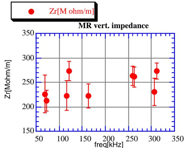
Figure 10: The vertical impedance of the Fermilab Main Ring from BTF measurements. The unit of y axis is in  $M\Omega/m$ .
