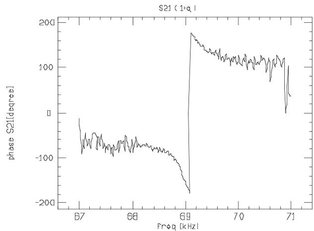
Figure 4: Phase of S21 (raw data) for the n=1+q sideband.
