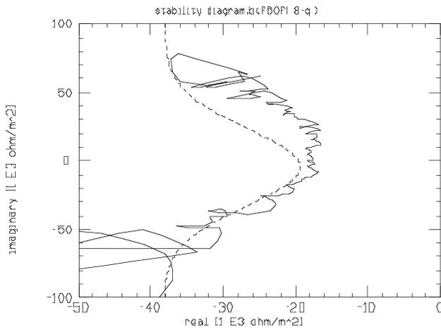
Figure 7: Stability diagram for the  $n=8-q$  betatron sideband.
