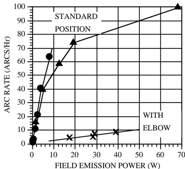
Figure 4. Arc rate as a function of additional power dissipated due to field emission for the same ceramic window with and without a waveguide elbow .
