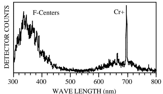
Figure 3. Optical emission spectra from an alumina sample irradiated with a 100pA, 30 keV electron source. The Cr<sup>+</sup> line is located at 694.1 nm.
