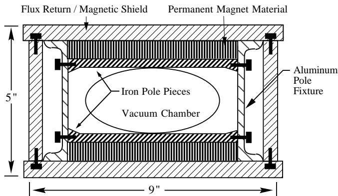
Figure 1: Cross-section of the 1 kG hybrid permanent magnet dipole. This design duplicates the Main Injector beam pipe dimensions and good field aperture ( $\pm 1.75"$  at  $\Delta B/B_0 = 10^{-4}$ ). The overall dimensions are 5"x9" and the weight of a 6 m section is approximately 2500 lbs. The field is driven by two permanent magnet blocks 3/4" thick by 6" wide.
