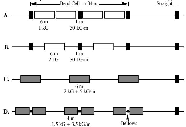
Figure 5: Sketch of the permanent magnet options under consideration in the magnet prototype program. Option A is a direct copy of the Main Injector lattice, while the 1.5 kG combined function option D is currently favored.
