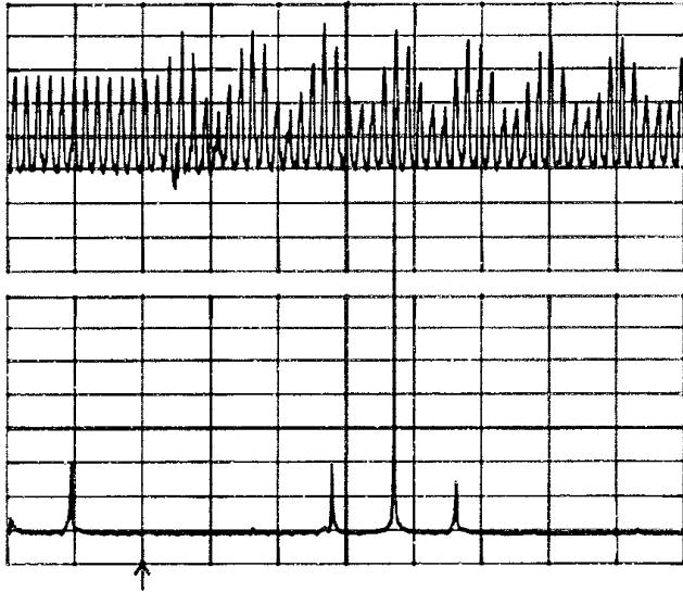
Figure 3. FFT of a broadband signal from the position monitor. Upper trace: pick-up signal, 10 \mu\text{s}/\text{div} . Lower trace: FFT of upper trace (RF-frequency and 3 betatron sidebands are shown), 100 kHz/div.
