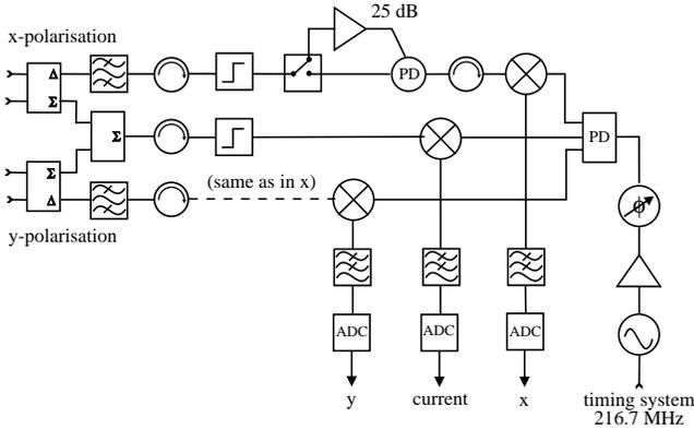
Figure 2. Signal processing scheme for the cavity BPMs
