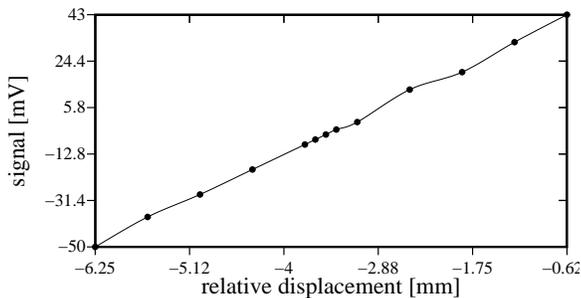
Figure 5. CTF-test - Output versus rel. position
