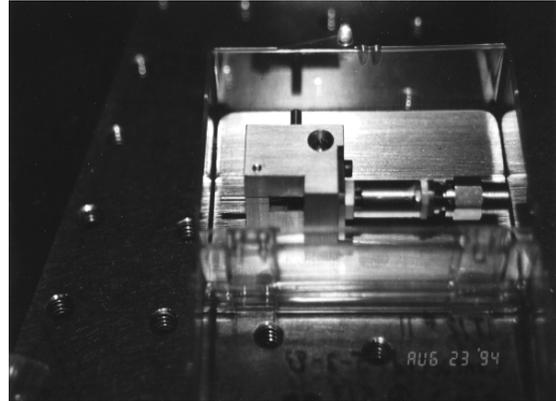
Fig. 2 Corner Cube and Schottky Diode Assembly
