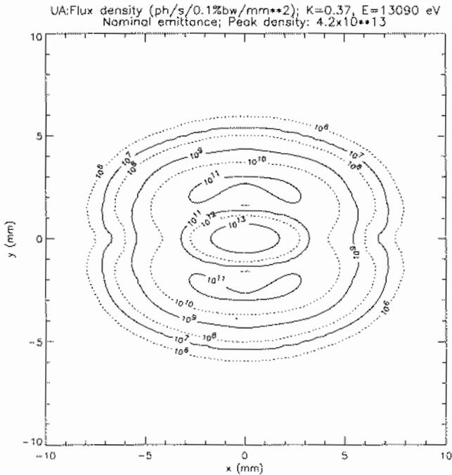
Figure 2: US calculation results in the undulator fundamental spectrum off axis in x and y. The intensity contours are indicated.
