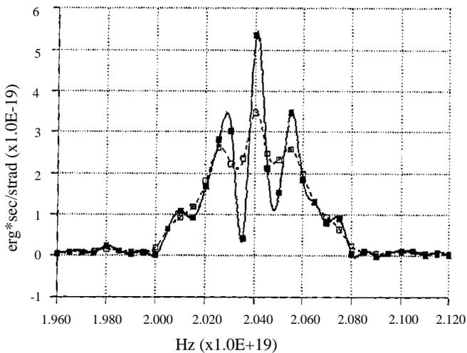
Figure 3: MDK1F results for an optical klystron configuration showing the calculated third harmonic spectral region without (solid) and with (dashed) 0.1% energy spread and no emittance.
