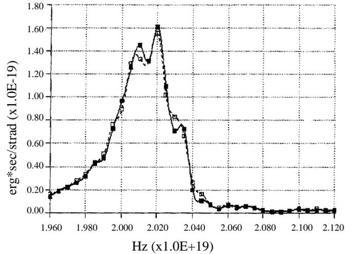
Figure 4: MDK1F results as in Fig. 3 with APS emittance effects added and with (solid) and without (dashed line) 0.1% energy spread.
