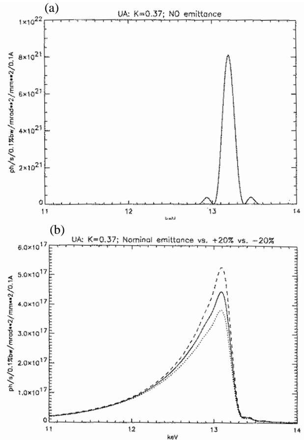
Figure 1: US calculation results for the undulator fundamental spectrum and with  $K=0.37$ : (a) zero emittance beam, and (b) an APS nominal emittance (solid line) and for  $\pm 20\%$  around the vertical emittance value.
