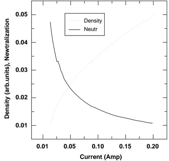
Fig.2. Neutralization factor  $\eta$  and density of ions  $n_i$  (in arbitrary units) versus beam current  $I$  (in Amperes),  $a = 0.05$  mm,  $B = 1$  Tesla,  $Y = 1$  m.
