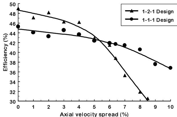
Figure 4. Simulated efficiencies of the first-harmonic output circuits.
