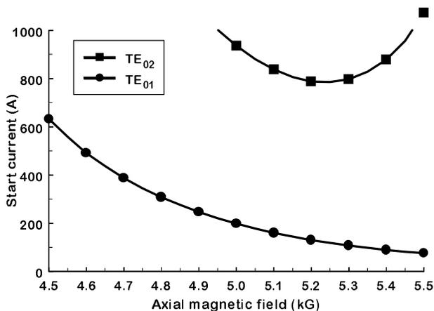
Figure 3. Start oscillation curve for the second harmonic buncher cavity.
