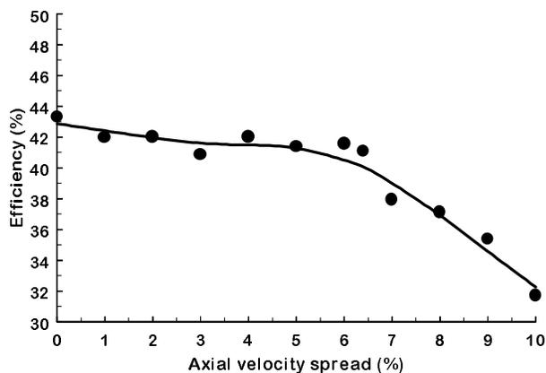
Figure 5. Efficiency of the second-harmonic output circuit.
