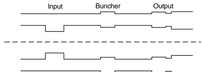
Figure 1. The second-harmonic output three cavity design.
