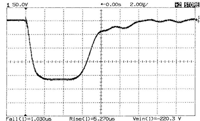
Figure 4: Improved Klystron Pulse
