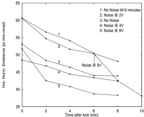
Figure. 2. Evolution of the horizontal emittance after a kick to measure the dynamic aperture
