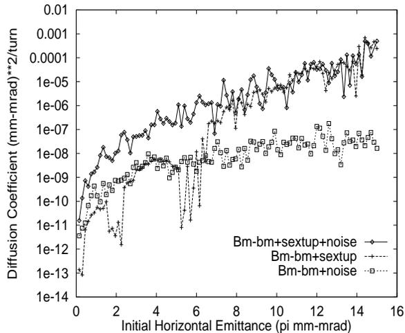
Figure. 3. Diffusion coefficient for the horizontal action calculated after a million turns for three cases. The noise correlation time  $\tau_c=10,000$ .
