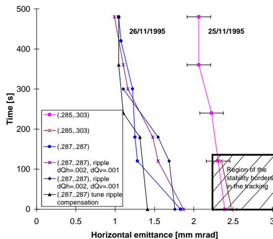
Figure 3. Horizontal Dynamic Aperture of HERA at Injection Energy Derived from Beam Profile Measurements. The box indicates the stability borders obtained by tracking calculations for small variations of closed orbit, ripple and strength of persistent current sextupoles.
