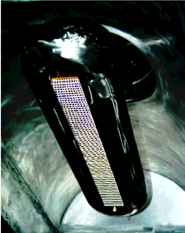
Figure 4. 10 cm by 100 cm flashover cathode assembly
