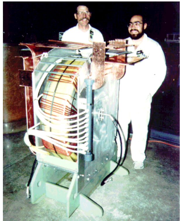
Figure 1. Fifth stage RHEPP 250 kV magnetic switch, with oil cooling manifold
