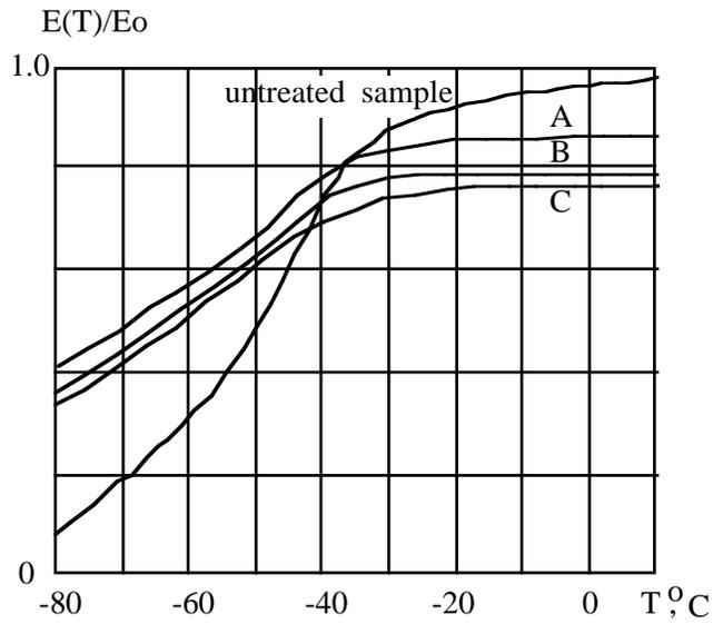
Fig.2. The silicone rubber (mark 914218, Caterpillar Inc.) module of elasticity  $E(T)/E_0$  relative change vs. temperature  $T$  for various values of an absorbed dose of electron beam irradiation (absorbed dose increases from sample A to sample C)
