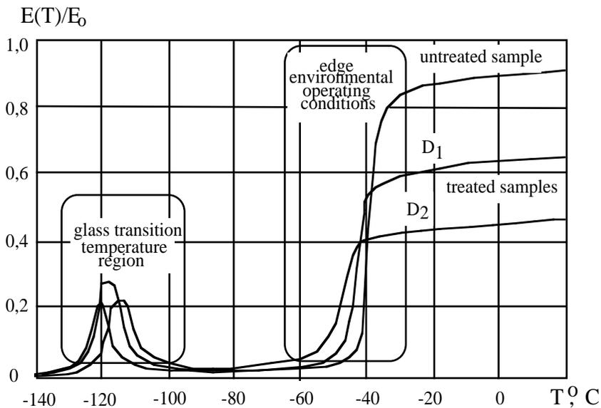
Fig. 1. The silicone rubber module of elasticity relative change  $E(T)/E_0$  vs. temperature  $T$  for various values of an absorbed dose ( $D_1 < D_2$ ).
