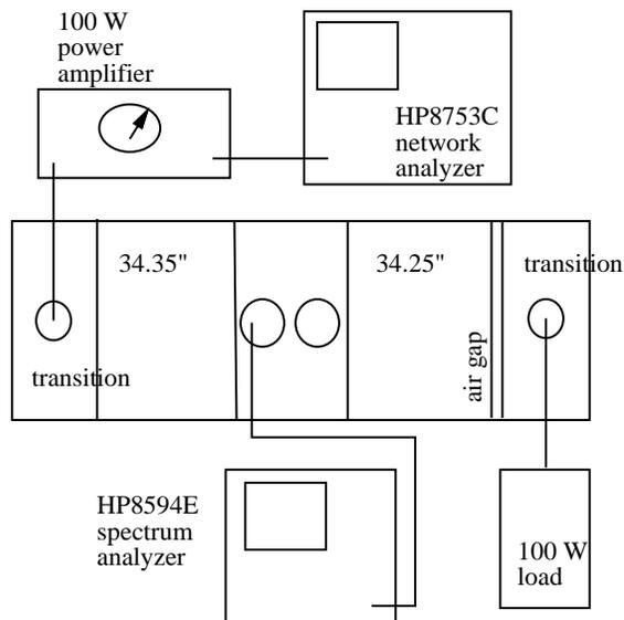
Figure 2. Measurement setup for the waveguide radiation test
