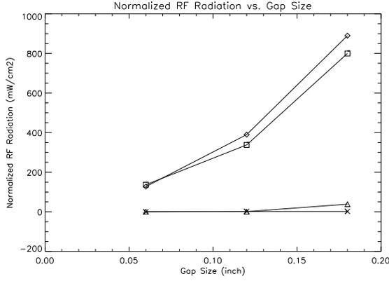
Figure. 5. RF radiation vs. gap size normalized to 100 kW input power
