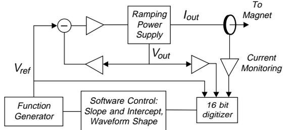
Figure 2: The present power supply control configuration.
