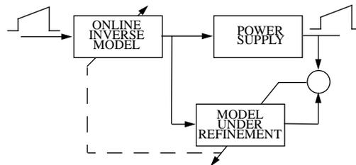
Figure 5: Adaptive Inverse Model Control Scheme.
