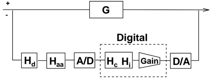
Figure 1. Block diagram of the ring and feedback loop showing the elements of the feedback system.
