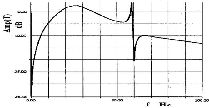
Figure. 5. Calculated amplitude response with notch filter.
