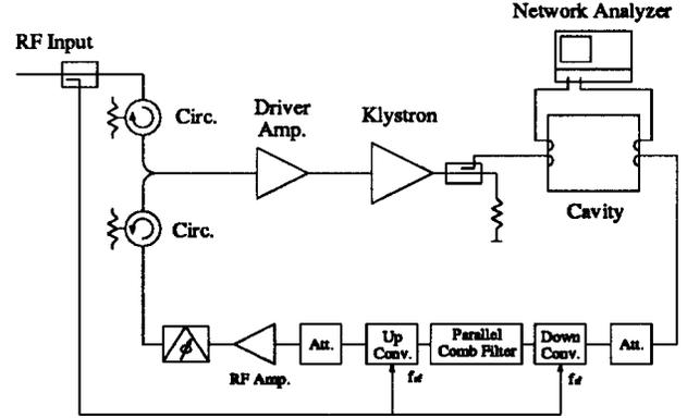
Figure 3. Block diagram of the experimental RF feedback loop which includes a parallel comb filter, a choke mode cavity and a klystron.
