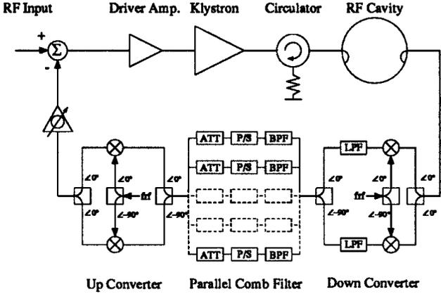
Figure 2. Block diagram of the RF feedback system using a parallel comb filter with frequency transposition by a single-sideband filter.
