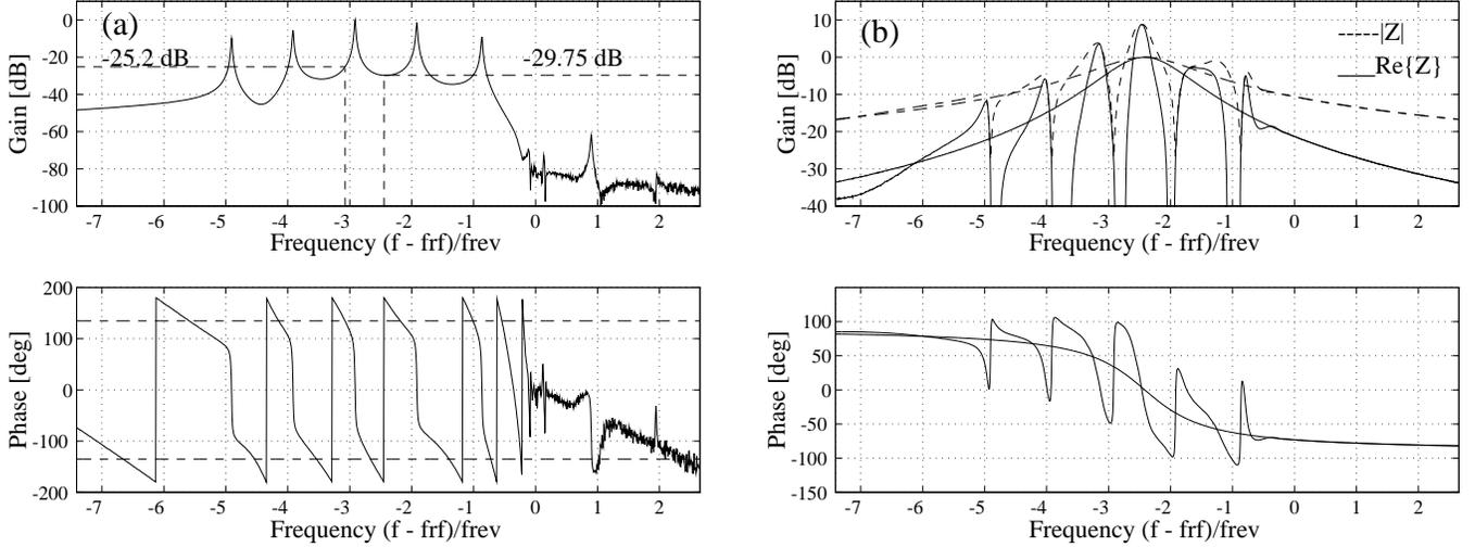
Figure 4. The measured open (a) and the closed (b) loop response as a function of normalized frequency  $(f - f_{rf})/f_{rev}$ .
