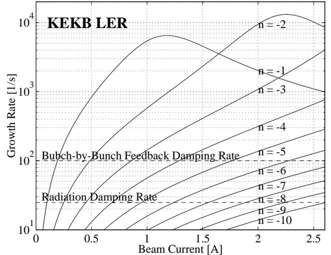
Figure 1. Estimated growth rate of longitudinal coupled-bunch instabilities due to the accelerating mode of choke mode cavities in the KEKB LER.
