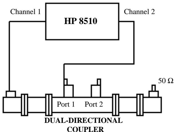
Figure 2: Measurement setup.
