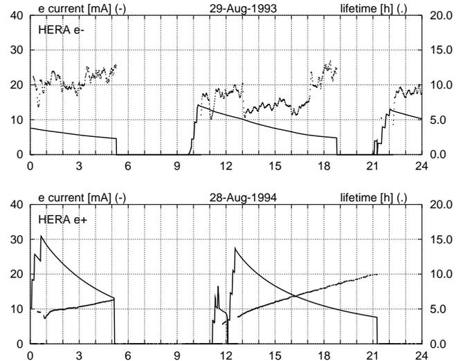
Figure 1. The current in mA (left scale) and and lifetime in hours (right scale) for a typical HERA  $e^-$  and  $e^+$  runs is shown. It is clear that the beam lifetime behaviour for electrons departs from that expected due to residual gas alone.
