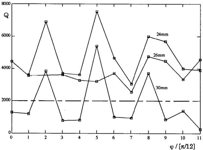
Figure 4: Measured Q-values of the first dipole passband.
