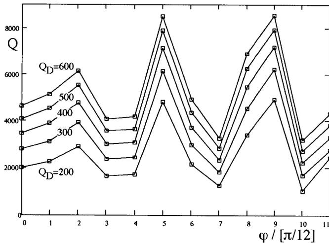
Figure 5: Calculated Q-values of the first dipole passband.
