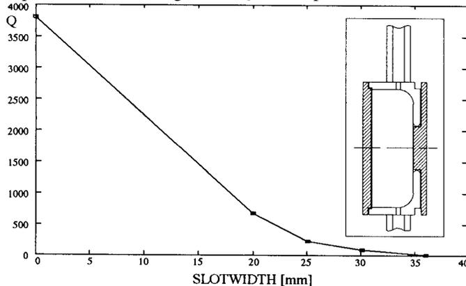
Figure 2: Single damper cell Q-value versus slotwidth.
