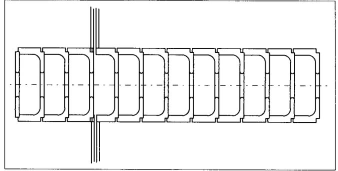
Figure 3: Damped 12-cell structure.
