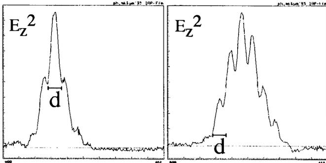
Figure 6: Measured Q-value of the  $11/12\pi$ -dipole-mode and related field distributions.
