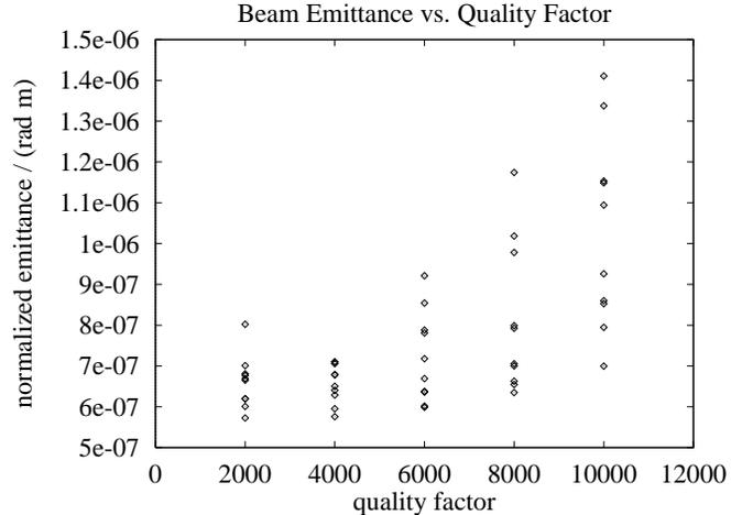
Figure 2. Normalized beam emittance at the end of the linac versus quality factor of the dipole modes. The acc. structures are moved with  $30 \mu\text{m}$  rms to the beam.
