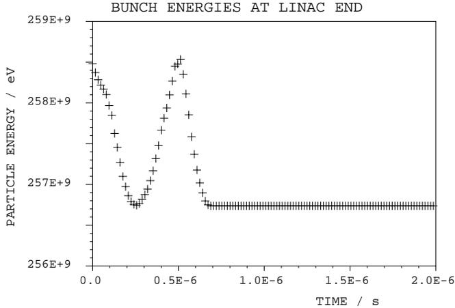
Figure 1. Compensation of the multi-bunch energy spread with staggered timing, results from computer simulations
