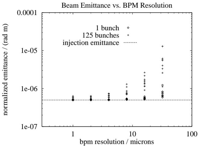
Figure 3. Normalized beam emittance at the end of the linac at single and multi-bunch operation versus BPM resolution. The dipole modes have a constant quality factor of  $Q = 2000$ . The acc. structures are moved with  $30 \mu\text{m}$  rms to the beam.
