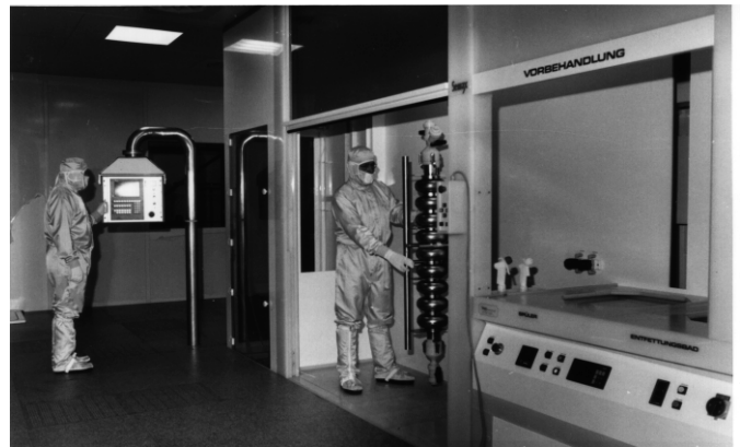
Figure 2: Cavity assembly in the clean room
