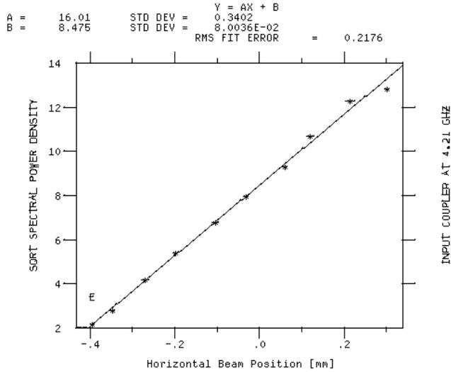
Figure 5: Structure BPM linearity measured at 4.21 GHz at the input coupler.
