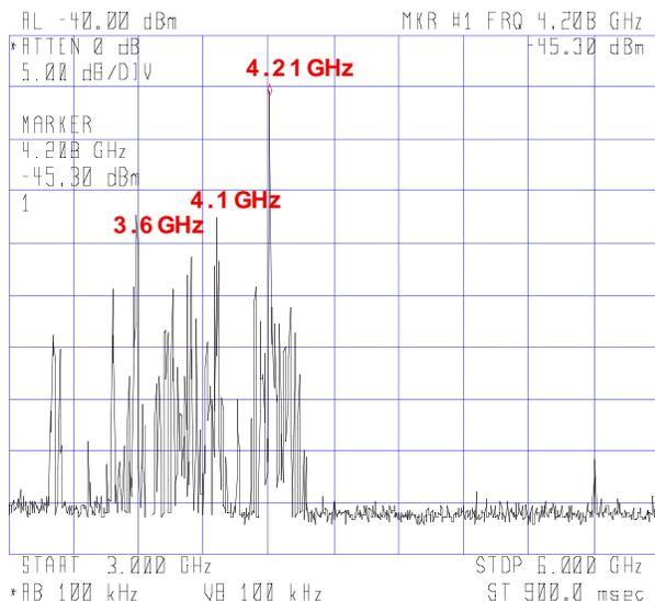
Figure 3: Beam-induced mode spectrum observed from the input couplers, measured from 3 to 6 GHz.
