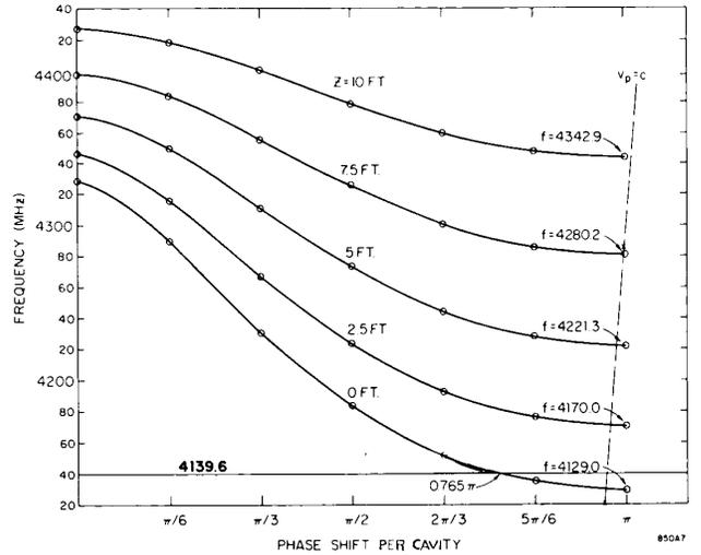
Figure 6: Dispersion diagram for dipole modes in the SLAC structure (reproduced from ref. 1).
