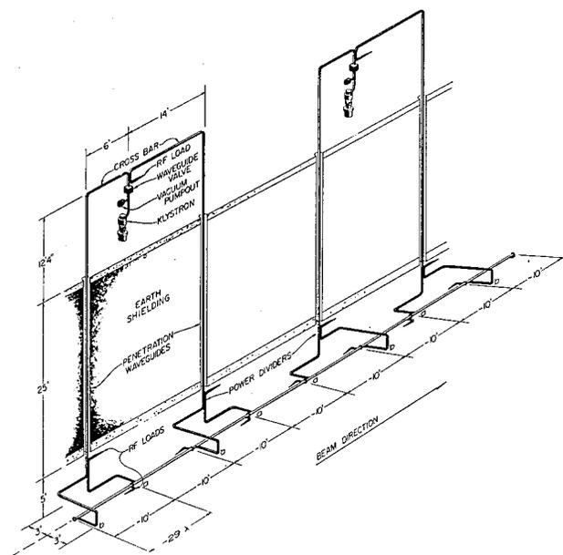
Figure 1: Layout of the accelerator and klystrons (reproduced from ref. 1). Signals were taken from the output load shown at the end of each 10' accelerating section, and from a coupler on the SLED cavity (not visible) located above each klystron.
