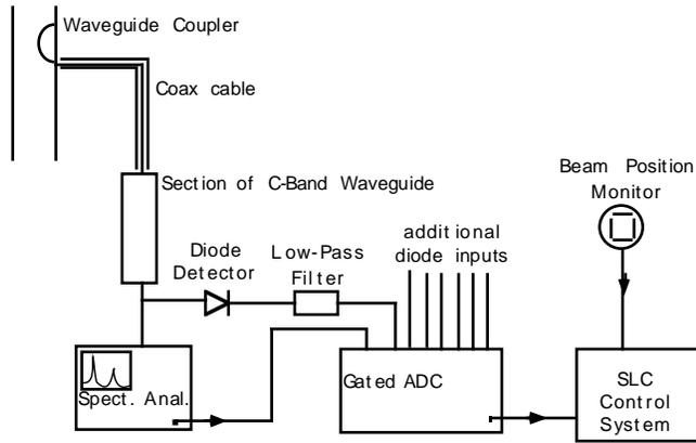
Figure 2: Layout of the instrumentation used for sampling the beam-generated modes in the structure. (not shown in detail in the figure) which is mounted above the klystron shown in fig. 1.
