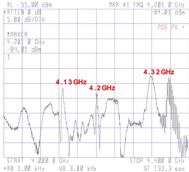
Figure 4: Beam-induced mode spectrum observed from the output couplers, measured from 4 to 4.4 GHz. also sampled by the GADC for similar correlation measurements. Although this signal is not as selectively filtered as the spectrum analyzer output, it does have the advantage of requiring much simpler instrumentation which can be duplicated to analyze the signals from several sections of waveguide at once.
