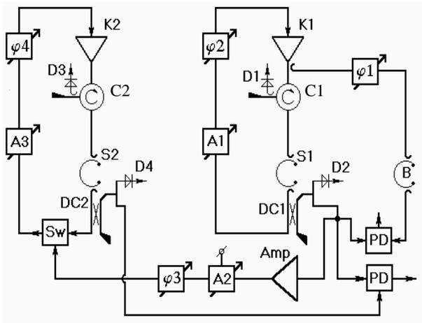
Fig. 2. Block-diagram of the accelerator RF system.
