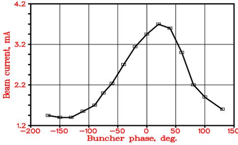
Fig. 4. Dependence of the output beam current on the buncher phase.
