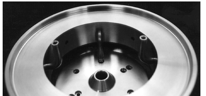
Photo 2 Close view of the disk-support-washer assembly
