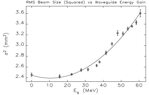
Figure 1. Bunch length measurement data consisting of  $\sigma^2$  vs  $E_g$ . The solid line shows the best fit quadratic curve to the data.
