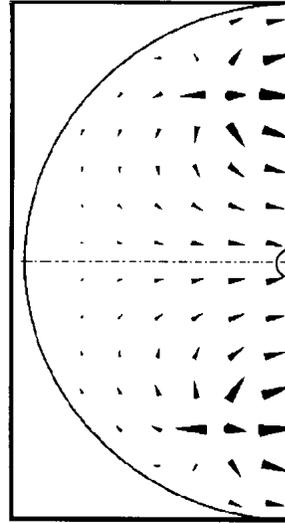
Figure 4. Magnetic field distribution in the centre of coupling cell for biperiodic on-axis coupled accelerator structure with one coupling slot per web.
