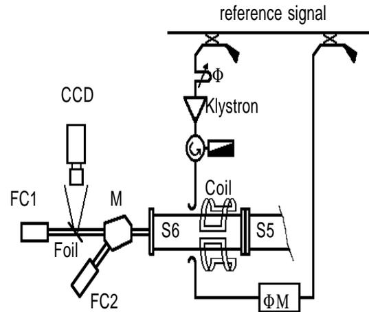
Figure 1. Schematic view (from the top) of the experimental set-up. Shown are: accelerator sections S5, S6, analysing magnet M, phaseshifter  $\Phi$ , phasemeter  $\Phi M$ , Faraday's caps, FC1, FC2, CCD TV camera, reference signal line, klystron, correcting coils.
