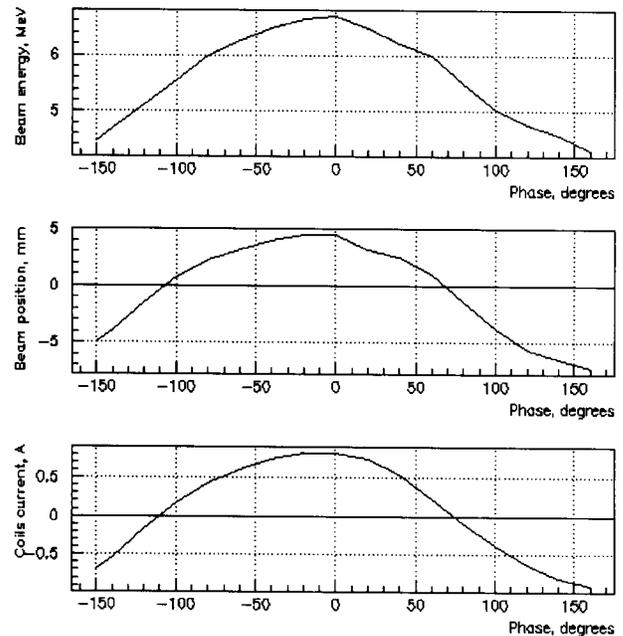
Figure 3. Dependence on the section 6 phase of beam energy (upper), beam position (middle), and correcting coils current (lower).
