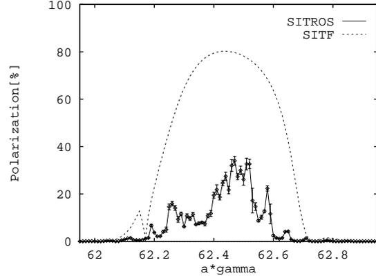
Figure 4. HERA electron ring without imperfections but with dispersion generating vertical bump at the beam-beam limit ( $\xi_z=0.04$ ).
