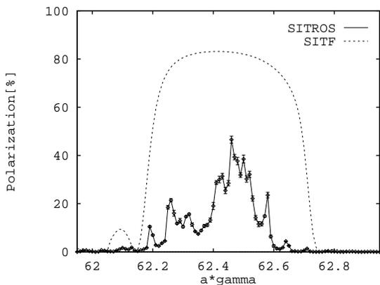
Figure 7. HERA electron ring with improved dispersion generating vertical bump with optimized spin harmonic content, at the beam-beam limit ( $\xi_z=0.04$ ).
