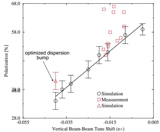
Figure 8. Polarization versus  $\xi_z$  for a machine with realistic distortions. Simulation (SITROS) results and measurements made in 1994 [1] are shown.
