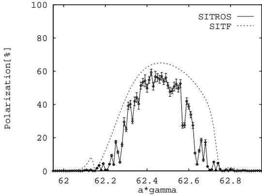
Figure 1. HERA electron ring with realistically modeled imperfections with a beam-beam tune shift of 0.01
