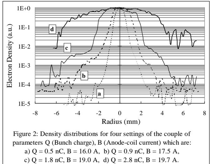
Figure 2: Density distributions for four settings of the couple of parameters Q (Bunch charge), B (Anode-coil current) which are:
