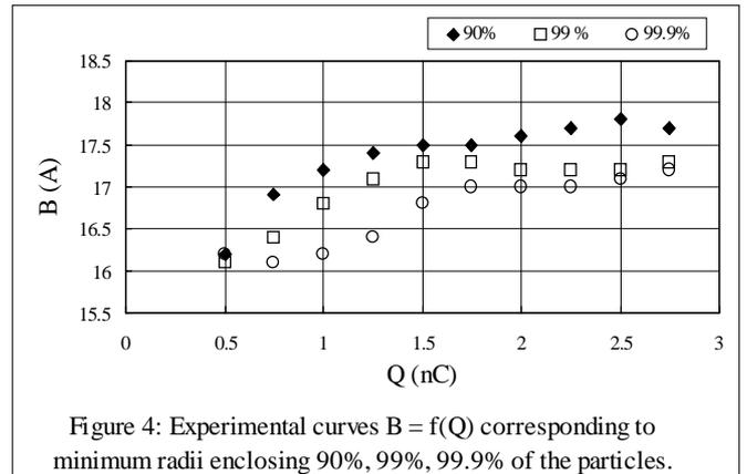
Figure 4: Experimental curves  $B = f(Q)$  corresponding to minimum radii enclosing 90%, 99%, 99.9% of the particles.
