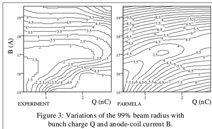
Figure 3: Variations of the 99% beam radius with bunch charge Q and anode-coil current B.
