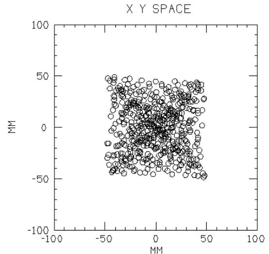
Fig. 2: Spatial distribution resulting from a non-KV injection.
