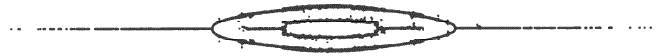
Figure 5. Simulation of a beam bunch, roughly 20 cm long and 0.2 mm in radius.
