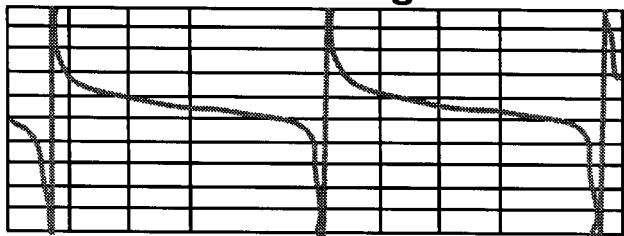
Figure 6. Response of IIR optical storage ring notch filter amplitude (top), phase (bottom). Center freq. 5 GHz
