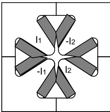
Fig.1. Asymmetric excitation of the arc quadrupole.
