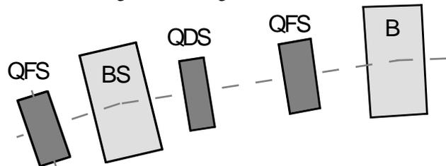
Fig.4 End-of-arc matching cell.
