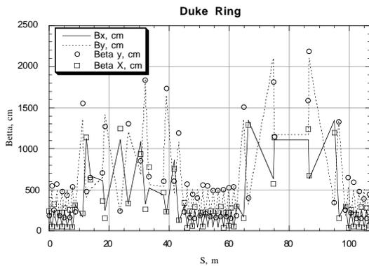
Fig.5 Measured and design values of  $\beta$ -functions.
