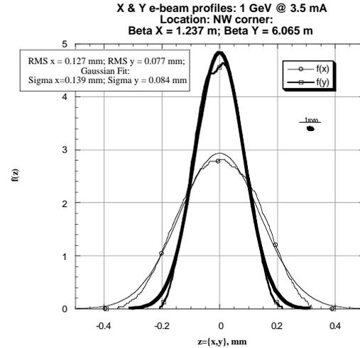
Fig.5 Measured e-beam profiles.
