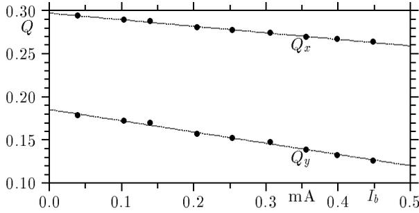
Figure 2. Measured tune change with bunch current
