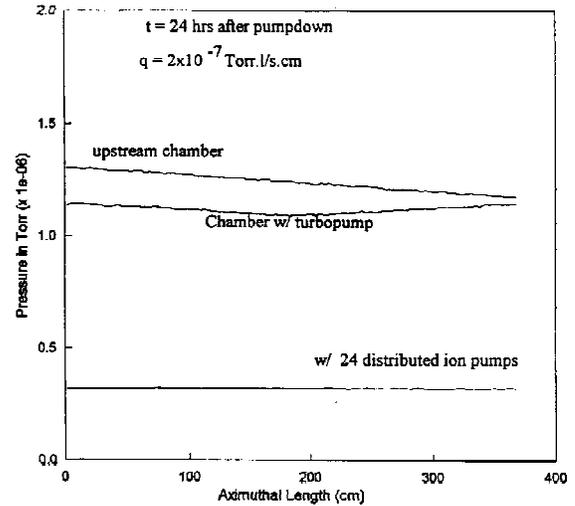
Fig. 6. Monte-Carlo simulation of pressure distribution inside the quadrupole electrodes using "Molflow" with 4 turbopumps; and with 24 distributed ion pumps. The x-axis represents the azimuthal length of the chamber. Total molecules generated in the simulation is approximately 30,000 per sector chamber.
