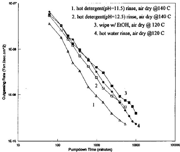
Fig. 5. Outgassing rates of the prototype sector chamber after various cleaning treatments. The designed outgassing rate of  $1 \times 10^9$  Torr.l/sec.cm<sup>2</sup> at  $t = 24$  hours can be reached with mild-etch detergent rinse.
