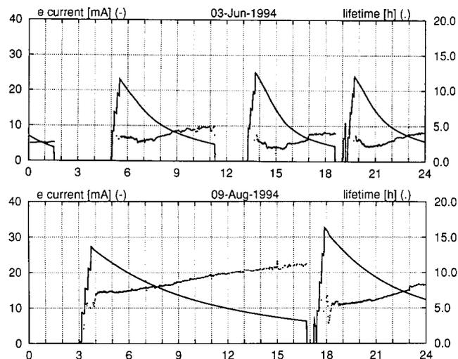
Fig. 3: Behavior of beam current (full line) and lifetime (dotted line, right hand scale) for typical electron fills (upper figure) and after switching to positron operation (lower figure).
