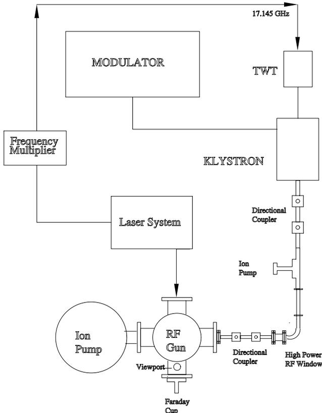
Figure. 2. Schematic of the experiment
