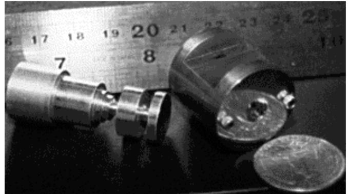
Figure. 1. RF Gun Cavity and Mandrel
