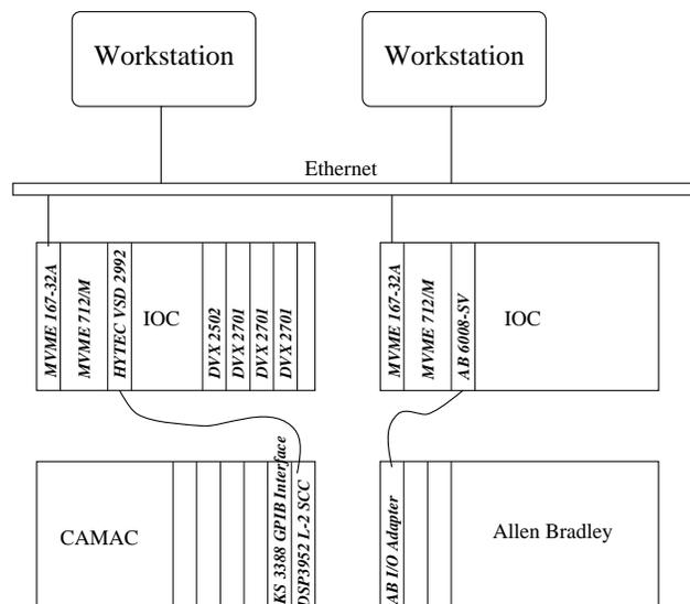
Figure. 1. Hardware layout for the Duke storage ring control system.
