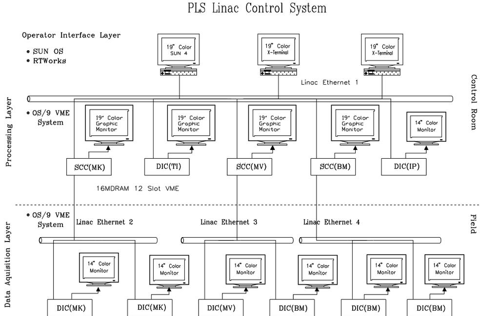
Figure 1: Schematic diagram for the PLS linac control system
