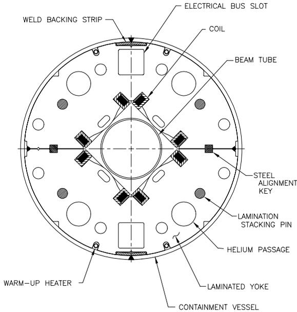
Figure 1. Cross Section of RHIC Trim Quadrupole.
