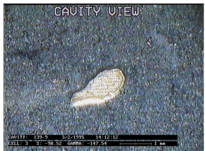
Fig.2: Inner cavity surface with 1.5 mm long irregularity.
