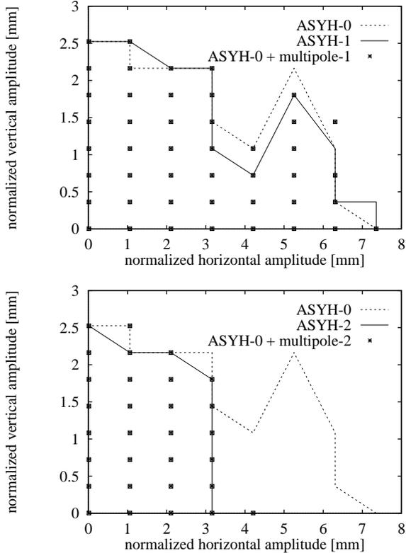
Figure 2. Stable amplitudes (normalized to  $\beta = 1m$ ) for the ASYH-1 (upper) and ASYH-2 (lower). The envelope of the stable amplitudes for the ASYH-0 is plotted as dashed line, for the ASYH-1 and ASYH-2 as solid line. The stable amplitudes for ASYH-0 and appropriate multipole lens (multipole-1 or multipole-2) are plotted as filled boxes.
