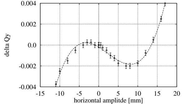
Figure 3. Measured tune shift with horizontal amplitude in the wiggler ASYH. The multipole coefficients obtained from the fit are  $b_2 = 1.0 \pm 0.25\text{T/m}$  and  $b_4 = -6000 \pm 1000\text{T/m}^3$ .
