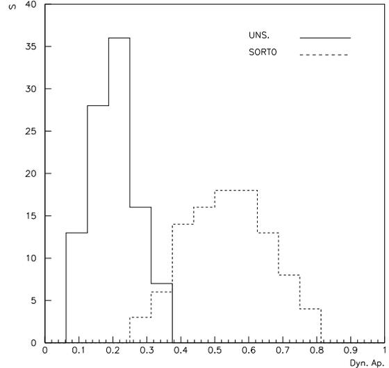
Figure 2. Comparison between the distribution of dynamic aperture for the unsorted machine and SORT0.
