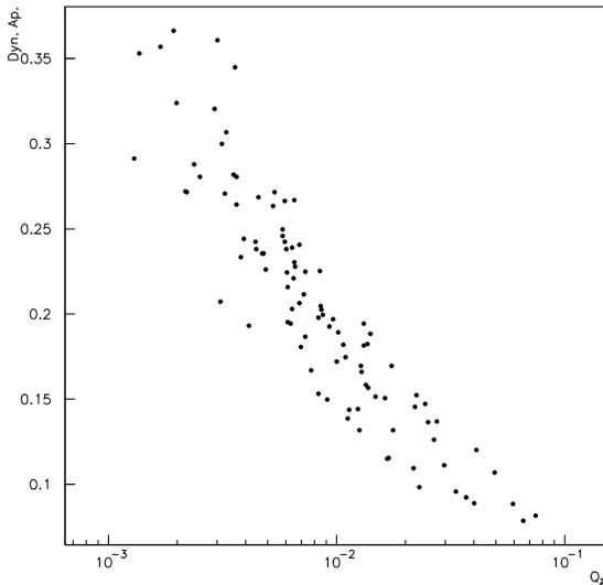
Figure 1. Correlation between the quality factor  $Q_2$  and the dynamic aperture for 100 seeds.
