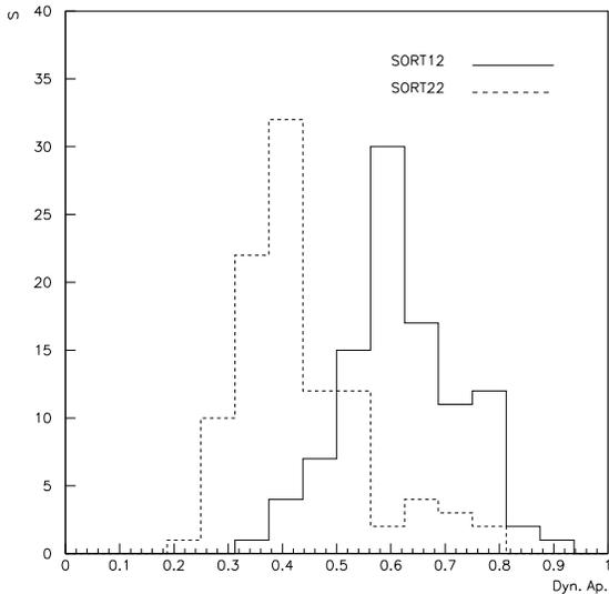
Figure 3. Comparison between the distribution of dynamic aperture for the SORT12 and SORT22.
